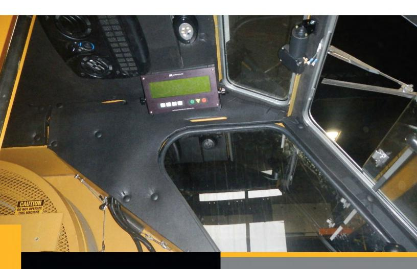
The new LMI systems will monitor crane configurations such as outrigger deployed, operating in high gantry or pile driving. They will also keep track of boom angle, load, rotation and superelevation.
